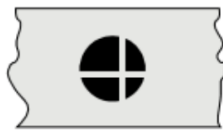
Fig. beam not centered
