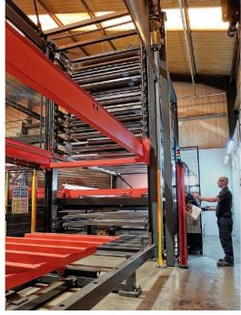
more than both of the previous CO2 machines combined. This performance is not only down to the speed of fibre laser cutting, but also because previous sheet replenishment, although automatic, was relatively slow. This task was achieved using swing-arm Byloaders to transfer material from pallets to the respective CO2 machines and offload the laser-cut sheets. Overall, utilisation of the machines was only 50 to 60%.
