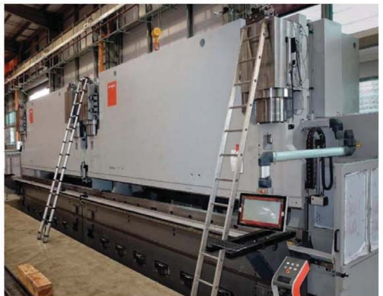
The tandem 650 tonne press braking facility being commissioned at Inishowen Engineering
