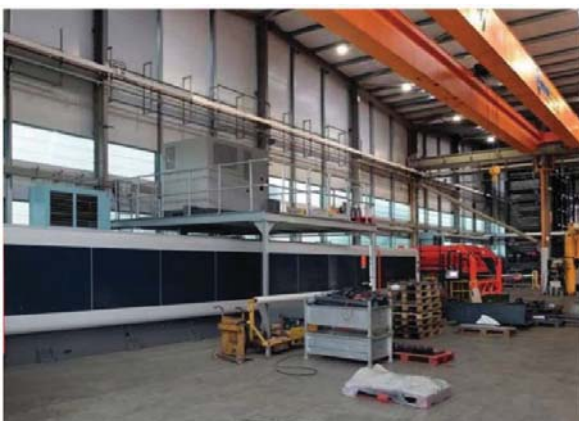
The Bystronic BySprint fibre laser cutting machine for processing 20m stock
