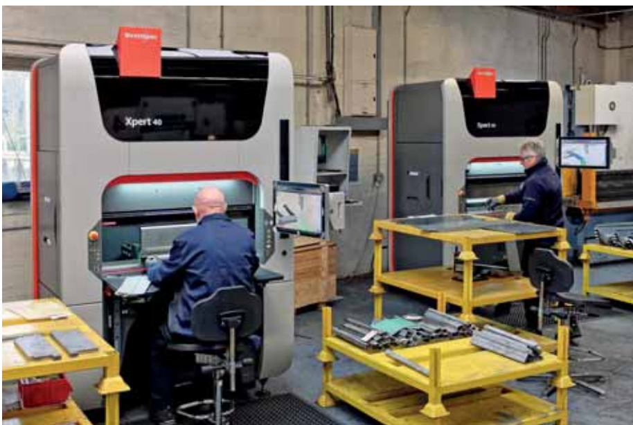
The pair of Bystronic Xpert 40 press brake cells in operation at Allsops. Almost all cut sheet metal at the Holmfirth factory is folded
