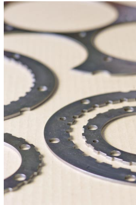
The Byjet cuts parts accurately within a tolerance of plus/minus one tenth of a millimeter.
