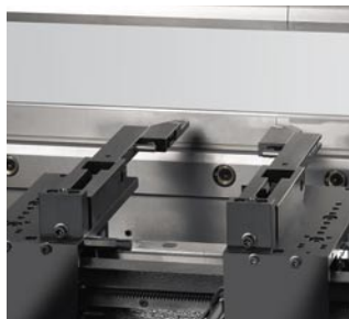
Type X, R: 2 DNC-controlled axes. Both fingers can be manually adjusted laterally in the Z plane.
