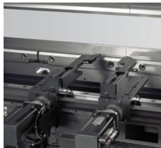
Type X, R, Z1, Z2: 4 DNC-controlled axes.
